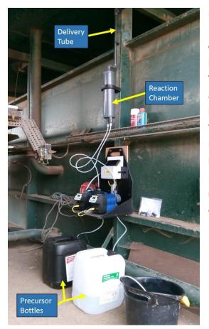
Scotmas Ltd undertook trials on Jack Buck Farms in Lincolnshire in July and August 2018. An automated dosing system, using precursor chemicals, was installed on one of the HWT tanks (pictured opposite). This uses a concentration monitoring system to achieve a set residual chlorine dioxide value which indicates that all pathogens have been destroyed. Trials were conducted over a period of two weeks until a steady residual level of CIO<sub>2</sub> could be maintained (in this case 1.6ppm).
